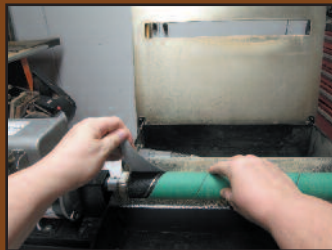
Velcro-backed sandpaper is wrapped around a drum inside a steel box.
