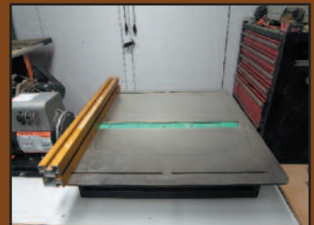
A steel table with a narrow gap is closed over the box and drum.
