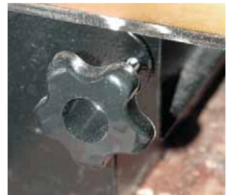
Photo.3: Table height micro-adjuster
