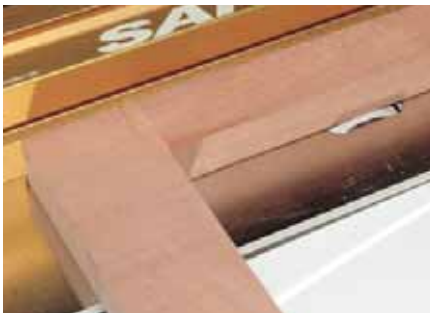
Photo.10: Finish sanding a frame
