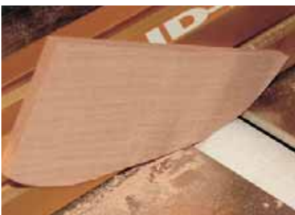
Photo.8: Sanding the edge of an outside curve
