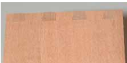
Photo.7: Dovetail box sanded with 120grit abrasive
