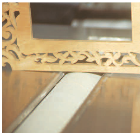
The table must be raised to eliminate the gap shown. The table is adjusted correctly in relation to the drum when NO gap exists between the wood and the table.
